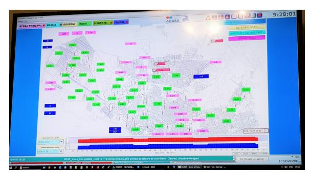
Figure 4. City of Brăila : Pink (metered/delimitated sectors), Blue (main pumping points of water into Brăila), green (pressure stations inside sectors and all over Brăila). Source: Dunarea 2019.
